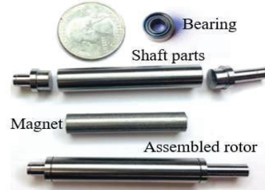
Fig. 22. Different parts and assembly of the optimized rotor (DP-2).
