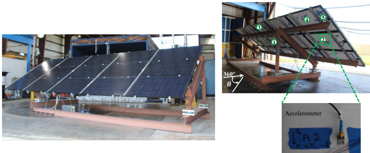
Figure 4. Full-scale PV array model and location of accelerometers at WOW EF.
