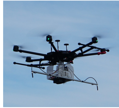
Fig. 3: The aerial node with the SDR and RF front end in the custom payload tray.
