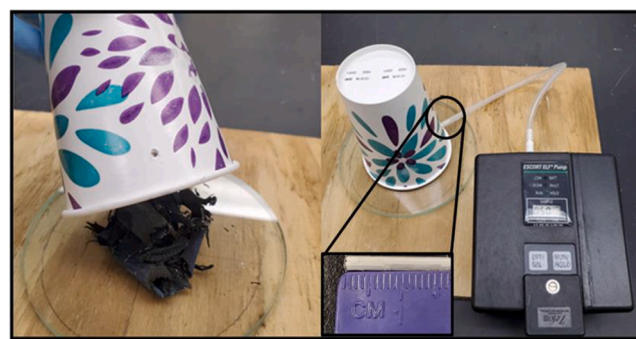
Fig. 1. Photograph depiction of the CMV/Cup apparatus with debris placed on the glass platform (left) and the CMV sampling using the hand-held vacuum pump (right).
