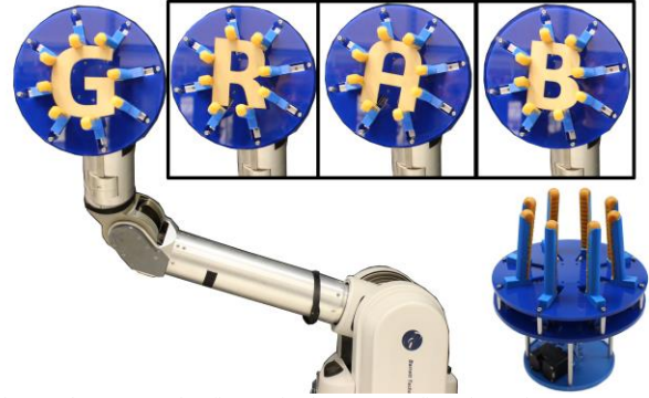
Fig. 1. The proposed 8-finger single-actuator fixturing gripper mounted on a robot arm and grasping planar lamina. Each finger translates radially inward until it comes in contact and exerts the same force on the lamina. Upon contact, the fingers lock passively and create a form closure grasp.
