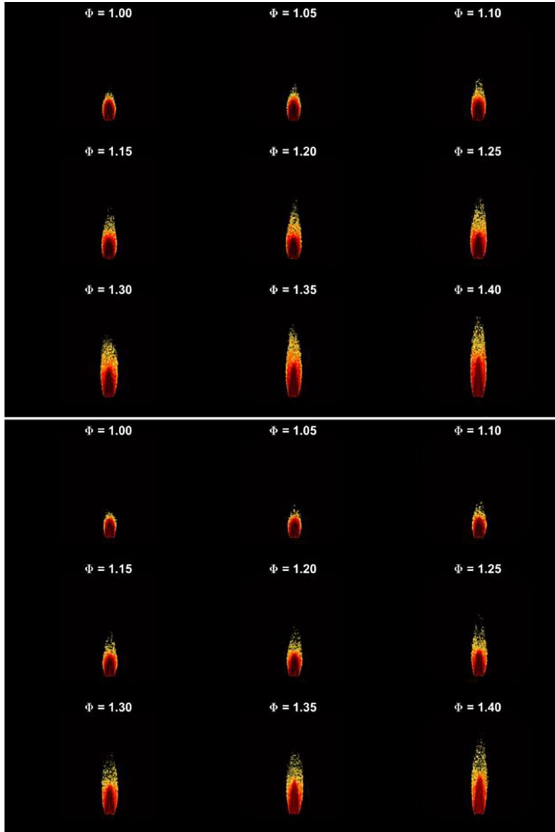
Fig. 6. 2D ratio images of recovered C_2^* /recovered CH^* for channel 1 (top) and channel 2 (bottom), indicating good fidelities for the recovered images from the multiplexed flame images.
