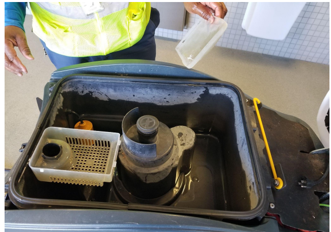
Figure 4: Image of a staff member cleaning the filter and refilling the tank of a floor scrubbing robot.
