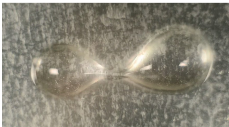
Figure 19. Glycerol drop on parafilm coated with a thin layer of a low-viscosity silicone oil and subjected to the voltage of 7 kV.
