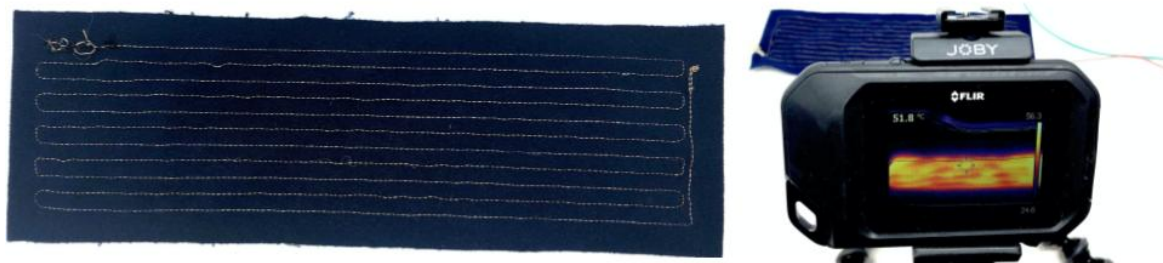
Figure 4: Stitches Thermal Element (left) and Thermal Image of Active Trace (right)
