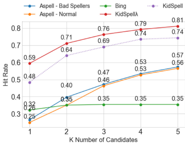
Fig. 6. Hit-Rate@k (where k is the number of provided suggestions) on the CHILDRENS MSP dataset. Note that the Bing Spell Check API only returns a maximum of 3 suggestions.
