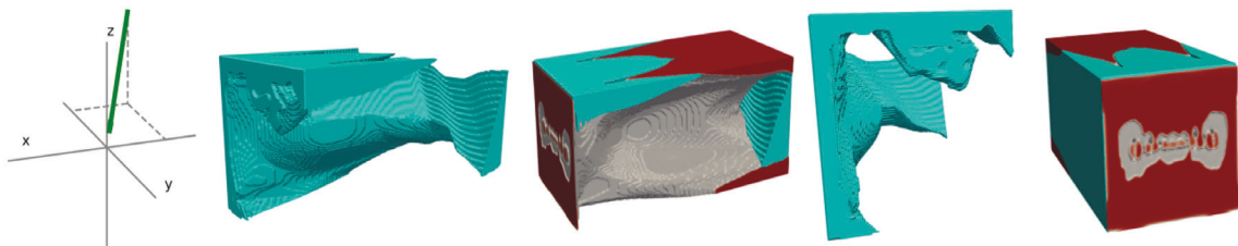
(D) \mathbf{a}_4 , two perspectives of the accessible volume of Figure 18(b) with respect to \mathbf{a}_4 , and two perspectives of these accessible volume exploded along \mathbf{a}_4 .
