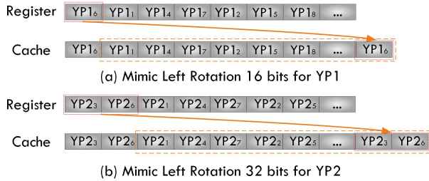
Figure 12: Rotation mimic mechanism
