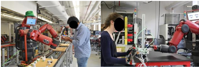
Figure 1. Two human-robot collaboration tasks performed in our Automation Lab. Left: A co-robot holds a deformable assembly base and the student mounts parts using a drill. Right: the student uses a pneumatic device to carefully level an assembly base, and the co-robot mounts small parts on this base. Given the nature of collaborative tasks, physically isolating the human workers from the co-robots is not applicable.
