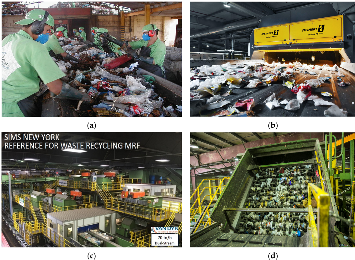
Figure 3. (a) Manual sorting process at MRFs, (b) automated sorting using optical sorter, (c) overview of an MRF sorting facility using multiple automated sorters, and (d) tangles as a key problem encountered by MRFs. Extracted from cleantechloops, steinertglobal, simsmunicipal, mydisposal.
