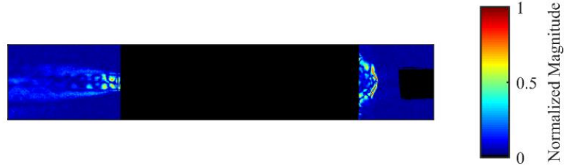
Fig. 9 Contour mapping of the relative intensity of the 20 kHz peak from Schlieren images
