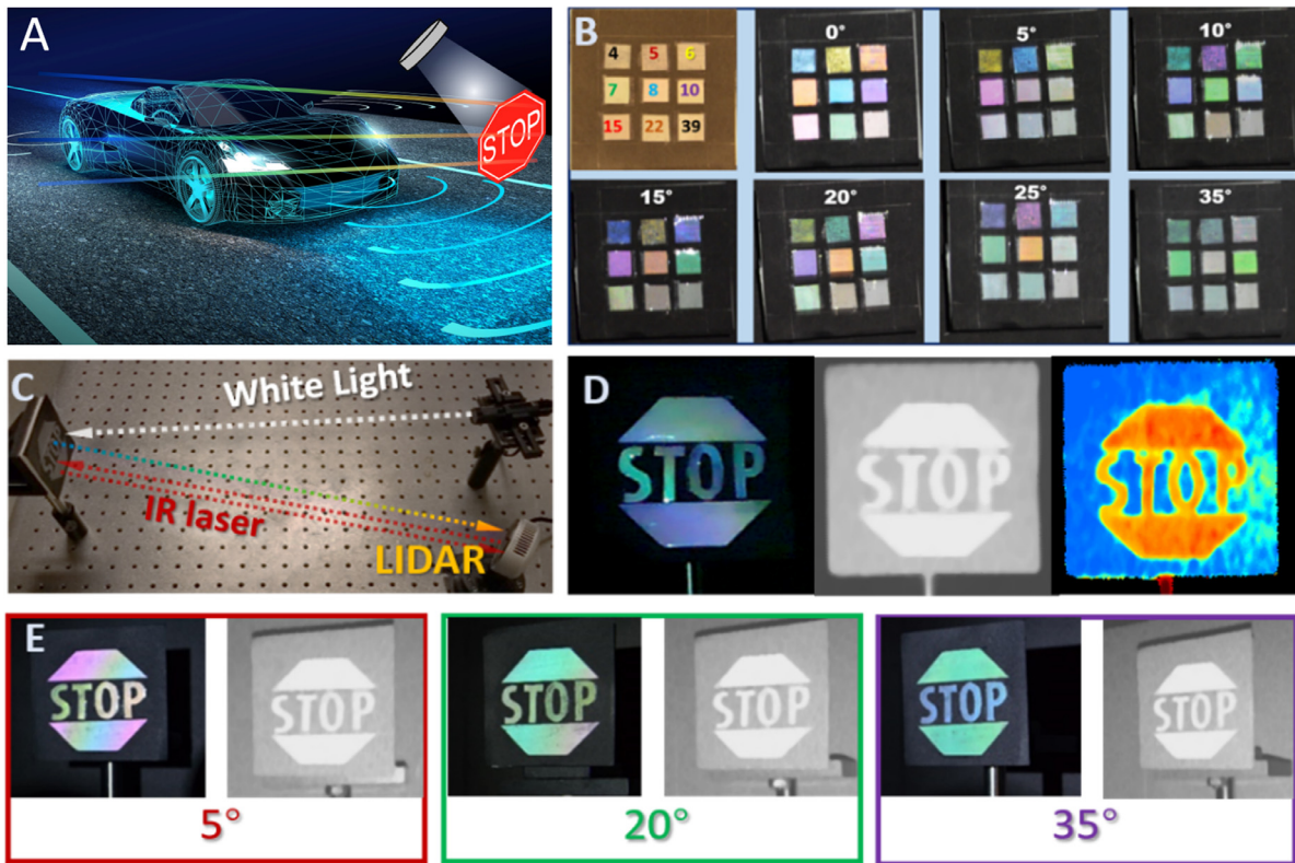
Fig. 6. Visible and IR reflective signs under different light illumination conditions. (a) Proposed implementation of MCI in LiDAR technology for simultaneous visible and IR imaging and pattern recognition. (b) A 3 \times 3 block of PS microsphere samples with various diameters (4, 5, and 6 \mu\text{m} in top row, 7, 8, and 10 \mu\text{m} in middle row, and 15, 22, and 39 \mu\text{m} on the bottom row). The observation distance is 20 cm. (c) Experimental setup used to demonstrate effectiveness of the MCI signs for indoor LiDAR application. (d) Simultaneous visible, IR and distance mapping images observed by the LiDAR camera at the normal direction and the distance of \sim 0.37 m. (e) Corresponding visible and IR images of the MCI sign observed at three different angles of 5^\circ , 20^\circ and 35^\circ , respectively (For interpretation of the references to color in this figure, the reader is referred to the web version of this article.).
