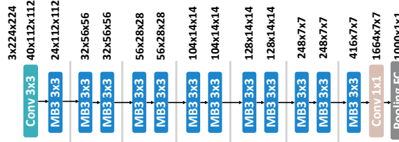
Fig. 2. An example architecture in the MobileNet-V2 search space, which achieves 70.2% accuracy on ImageNet and 71ms average inference latency on S5e. The text “ Z_1 \times Z_2 \times Z_3 ” the input size for each layer.
