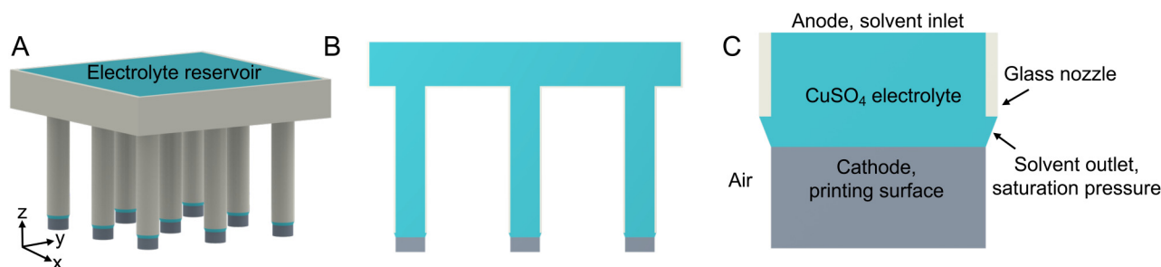
FIG. 1. (a) A CAD rendering of the 3 \times 3 nozzle array, (b) a cross-sectional view of the array, and (c) a close-up view of a single nozzle tip with the applied boundary conditions. The same boundary conditions were applied to all nozzles. The contours for the meniscus surface and meniscus height are shown in Fig. S1 in the supplementary material .
