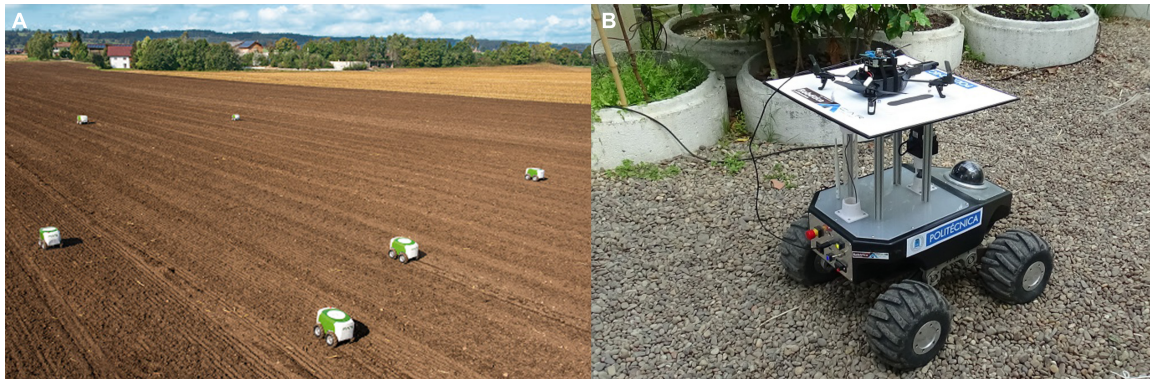
FIGURE 5 | (A) Mobile Agricultural Robot Swarms (MARS) for seeding process (The European Coordination Mobile Agricultural Robot Swarms (MARS). PDF file. November 11, 2016. http://echord.eu/public/wp-content/uploads/2018/01/Final-Report-MARS.pdf ), (B) UAV-UGV cooperative system to measure environmental variables in greenhouse (Roldán et al., 2016).
