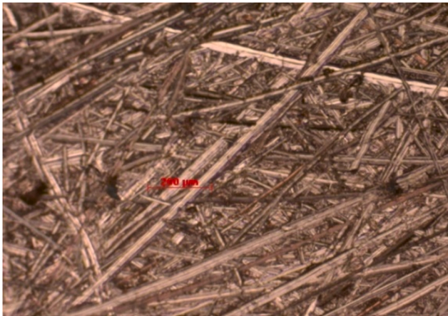
Fig. 20b. Optical microscope picture of the bare copper surface with surface modification using sandpaper.
