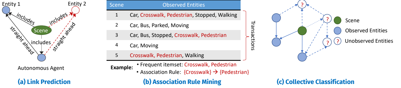
Fig. 3. Three possible solutions devised for KEP based on different machine learning/data mining techniques
