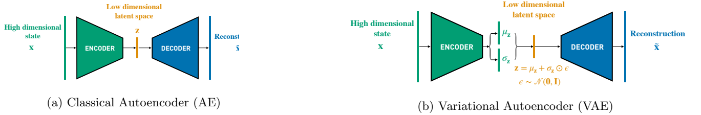
FIG. 1: (a) A schematic diagram of a classical Autoencoder (AE). A high-dimensional state \mathbf{x} is mapped to a low dimensional feature space \mathbf{z} by applying the encoder transformation through multiple fully connected layers. The low dimensional feature space \mathbf{z} is expanded in the original space by the decoder. The autoencoder is trained with the loss \mathcal{L} = \|\mathbf{x} - \tilde{\mathbf{x}}\|^2 , so that the input can be reconstructed as faithfully as possible at the decoder output. (b) A schematic diagram of a Variational Autoencoder (VAE). Instead of modeling the latent space deterministically, the encoder outputs a mean latent representation \mu_z , along with the associated uncertainty \sigma_z . The latent space \mathbf{z} is sampled from a normal distribution \mathbf{z} \sim \mathcal{N}(\cdot | \mu_z, \sigma_z \mathbf{I}) , with diagonal covariance matrix.
