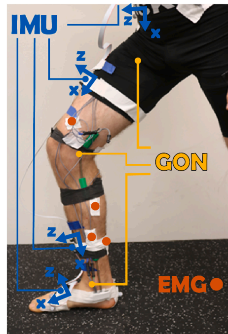
Fig. 1. Sensor placement. EMG electrodes were placed on the lower limb, targeting the major muscle groups. Goniometers were placed at the hip, knee, ankle. IMUs were placed on each segment of the lower limb and the torso.
