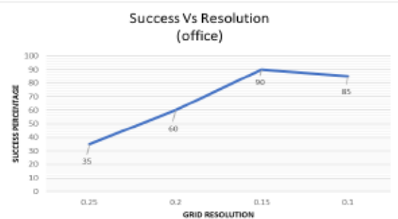
Fig. 13. The figure shows the impact of grid resolution on the performance of the algorithm. 20 trials were conducted per grid resolution.
