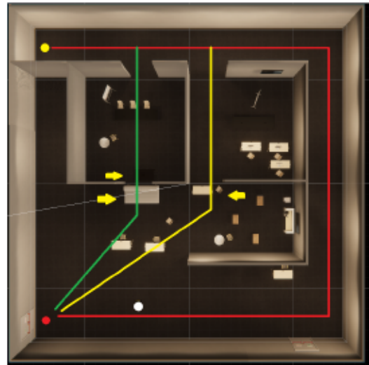
Fig. 4. The figure shows an overhead view of our office environment. The yellow dot indicates the human evacuees spawn point. The white dot indicates the robot start position. The red dot indicates the exit point. The red line is a longer path taken by the evacuees to the exit and was always unobstructed whereas the green line represents a shorter path taken by the evacuees once the blocking obstacle was removed. The yellow line is an intermediate path taken by the evacuees after the successful removal of the obstacle. The yellow arrow shows the obstacles to be moved.
