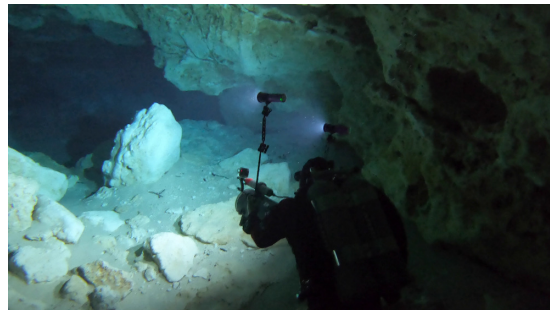
Fig. 1: Collecting data in an underwater cavern, Ginnie Spring, FL, USA. GoPro 9 camera is attached to the stereo-rig [15], lighting from two Keldan lights [16].
