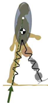
Fig. 1. Depiction of Virtual Pivot Point (VPP) model overlaid on top of a human walking with an Open Source Leg (OSL) prosthesis.
