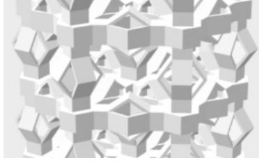
Figure 8: Hexagonal triangulated lattice with Sarrus ribs, oblique view.
