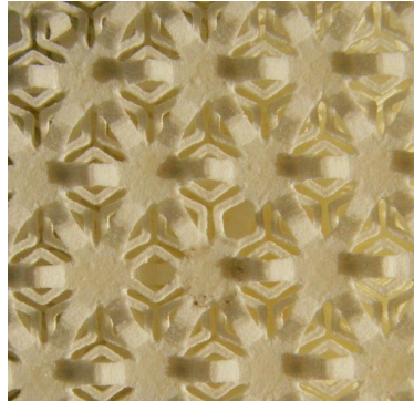
Figure 7: Hexagonal triangulated lattice with Sarrus ribs, transverse plane.
