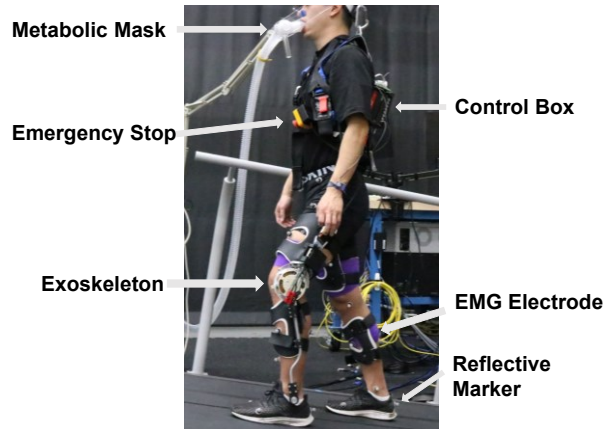
Fig. 3. Experimental setup during incline walking. The orthotic interfaces and the location of the actuator were adjusted to each subject's legs.
