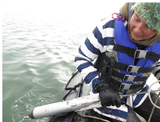
Figure 2. Portable free-fall penetrometer BlueDrop during YUKON14 deployments.
