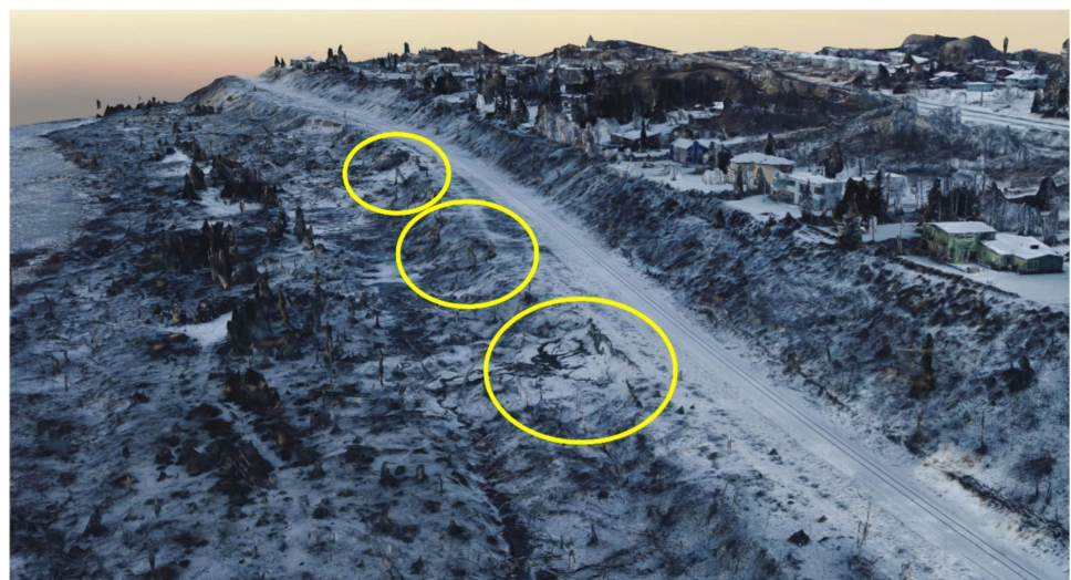
Figure 3. UAV-based 3D SfM reconstruction of an Arctic coastal slope near Anchorage that was impacted by an earthquake and landslides in 2018 (localized landslides are circled in yellow).
