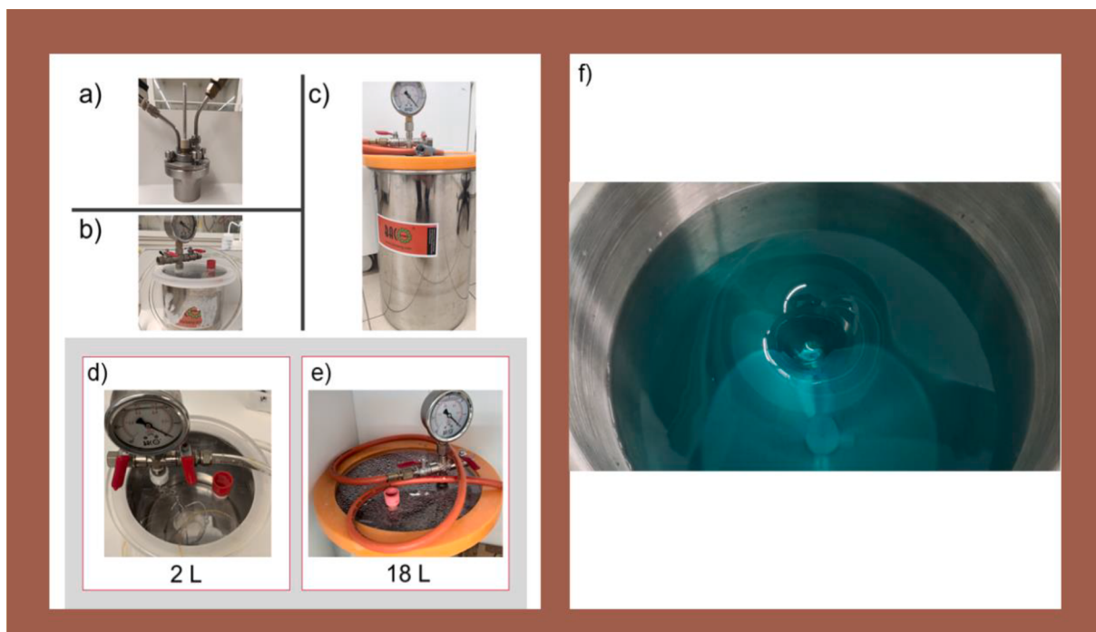
Fig. 1. Digital pictures of a) 50 mL, b) 2 L and c) 18 L reactors; heads of the (d) 2 L and (e) 18 L reactors; f) the 18 L reactor loaded with the polymerization mixture for the 15 L seATRP of AAm (see Table 3 entry 6).
