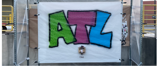
Fig. 1. Our system captures artist painting motions of individual letter outlines which are composed and processed into controls for a cable robot to execute. Our system produced this painting of the letters “ATL” (Atlanta).
