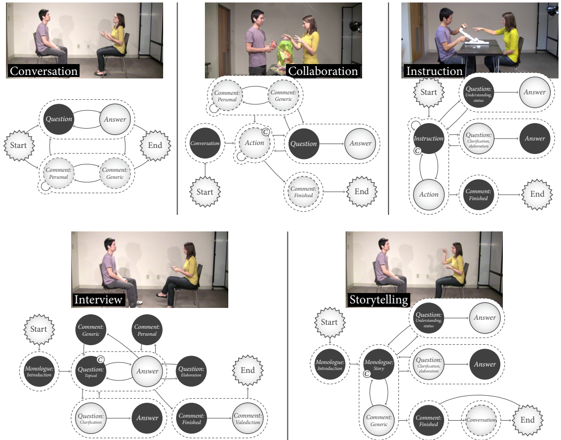
Figure 2. Five HRI models [18] derived from dyadic human-human interaction data. Each model contains start and end states. Dark and light gray states represent one or the other agent in the dyad. States with dotted outlines can be enacted by either agent. Larger dotted regions correspond to the patterns uncovered by Sauppé and Mutlu [17]. A “C” is placed over components that are core to the interaction scenario.
