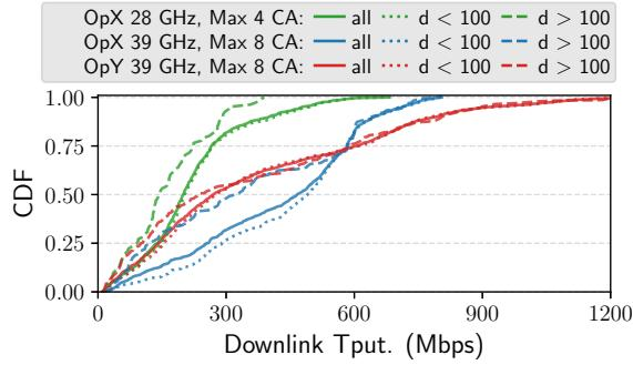
Fig. 12: Throughput comparison for different distances in DT.
