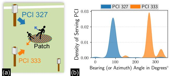
Fig. 9: OpX: UE @ BP prefers PCI (and Beam) with LoS.
