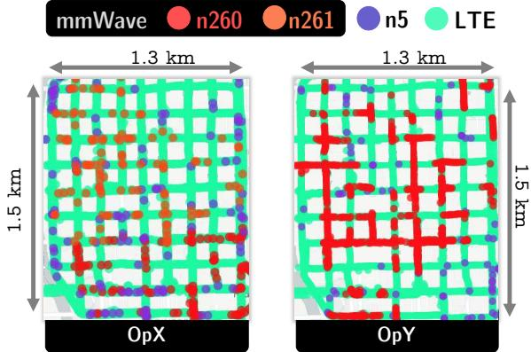
Fig. 3: Outdoor mmWave coverage around Chicago Loop area.
