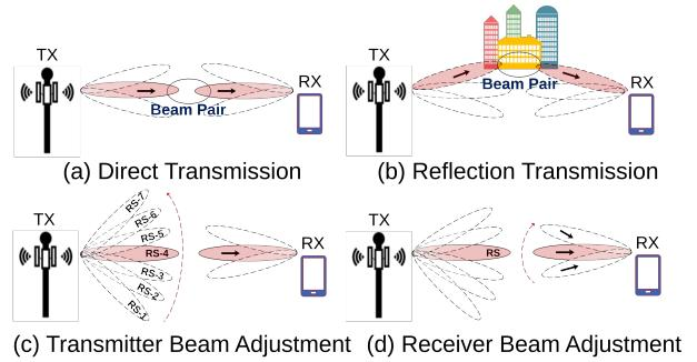
Fig. 1: Beam Management in 5G NR mmWave
