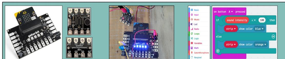
**Data Sensor Hub (DaSH):** The gator:bit is an extension of the micro:bit which exposes more pins for alligator clippable sensors that measure temperature, soil moisture, sound, humidity, CO<sub>2</sub>, etc. It provides functionality for simple data displays using LEDs and a speaker. Students program the micro:bit using MakeCode.
