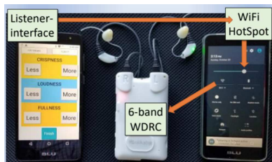
Figure 8: Apparatus used for the SFP study. The arrows represent the information flow from the listener interface, via WiFi, to the Portable OSP to tune the WDRC.
