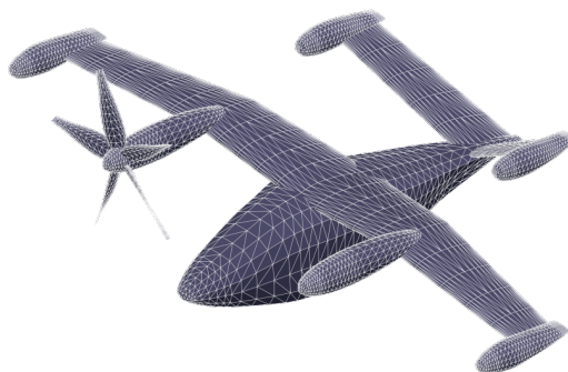
Fig. 6. Joby S4 UAM eVTOL vehicle with a single operating 5-bladed propeller in forward-flight mode (Case 1).
