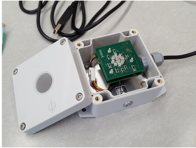
Fig 38 Photograph of one of three LED flashers currently installed in the pSCT. The cover containing the diffuser is open to expose the LEDs and circuit inside the module. The flasher enclosure is 8 cm x 8 cm x 5.5 cm and the diffuser lens has a diameter of 2.5 cm
