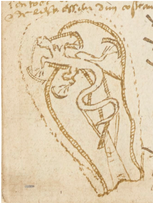
Fig. 1 Ms. Fr. 640, fol. 124v, Bibliothèque nationale de France, Paris. Drawing of the mold of a life-cast lizard. The gate of the mold allows metal to enter the lizard's tail, with sprues carrying the metal throughout the mold. Vents run from the lizard's head to allow air forced out by the intruding metal to exit through the gate end of the mold. Photo: gallica. bnf.fr.
