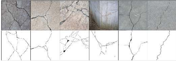
Fig. 3. Illustration of raw crack images and the annotated binary images in CSSC dataset.
