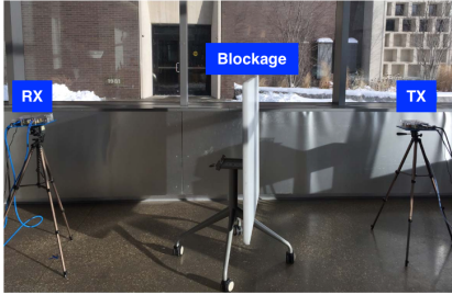
Fig. 8: Experimental setup showing LOS blockage with a wooden table.
