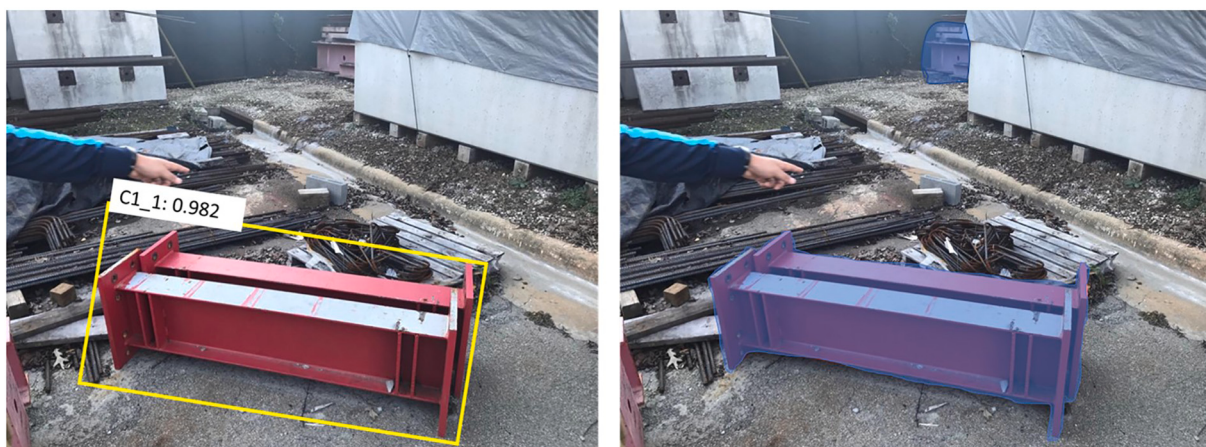
Fig. 5. Object Recognition output examples: a) Bounding Box b) Instance Segmentation.
