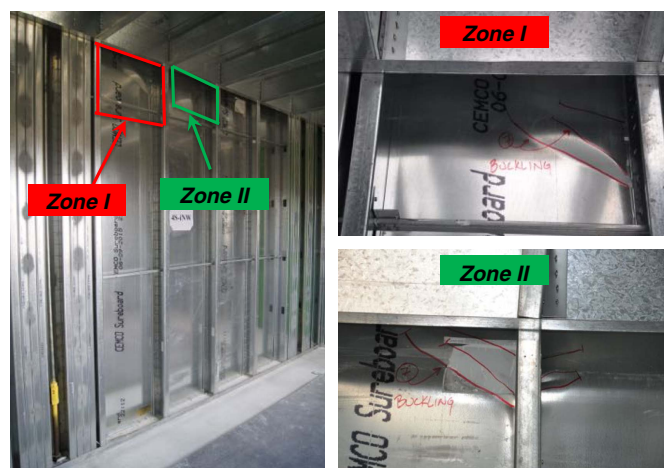
Fig. 9. Structural sheathing sheet steel local buckling of the Level 4 corridor shear wall at the end of the prefire earthquake test phase. (Images by Xiang Wang.)
