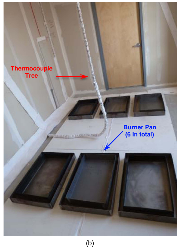
Fig. 4. Fire test protocol: (a) location of the fire compartments overlaid within the building plan layout; and (b) compartment fire test setup (southwest room at Level 2, Fire test 1) (image by Praveen Kamath).
