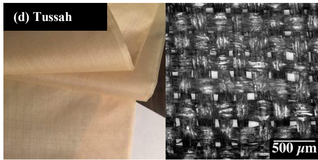
Figure 1. Silk fabric and corresponding macro- and micro-architectures: (a) Ahimsa silk, (b) Charmeuse silk, (c) Habotai silk, and (d) Tussah silk architectures. Left: macroscopic silk fabric images. Right: microscopic images of silk architecture at 50X magnification.
