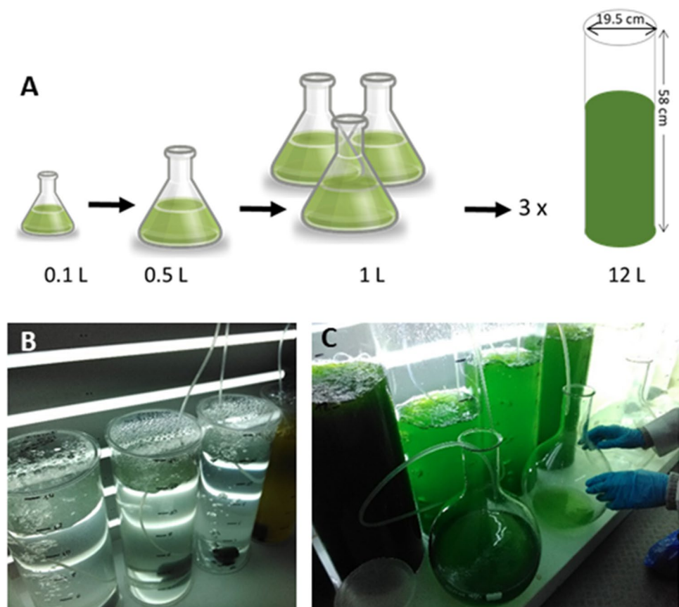
Fig. 1 (A) Diagram showing the scaling up procedure during the experiments; (B) Tubular photobioreactors (PBRs) used in the experimental set-up on day 0. (C) PBRs during sampling during exponential growth phase
