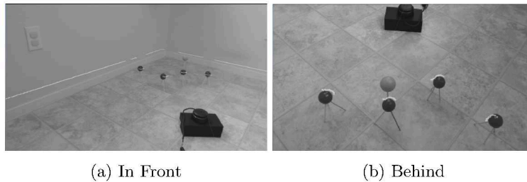
Fig. 8: Camera above the laser plane observing the calibration target from the front (a) and behind (b) with laser visualization applying our method’s calibration result.
