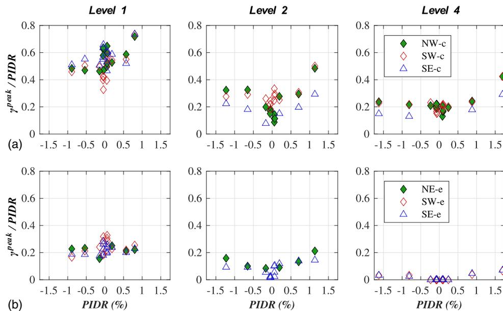
**Fig. 9.** Normalized peak panel shear distortions of the (a) corridor; and (b) corner shear walls during the prefire earthquake test sequence.
