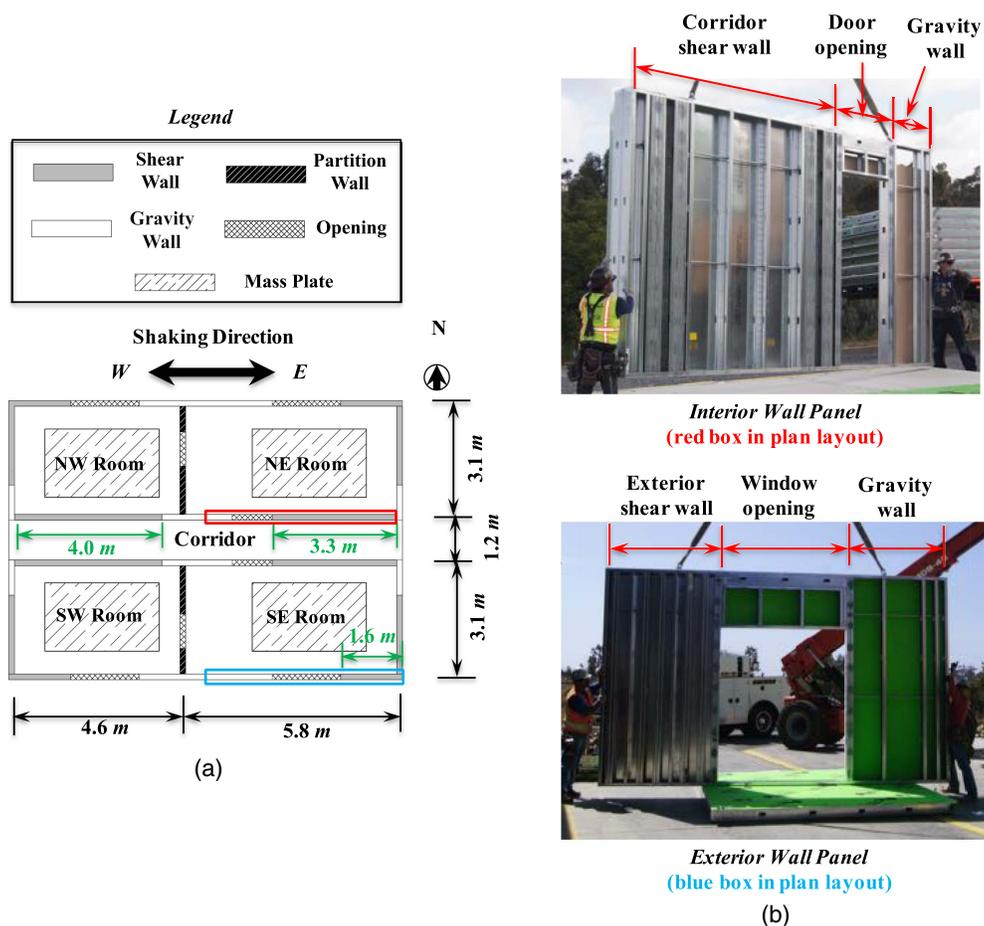
**Fig. 1.** (a) Test building plan layout representative of Levels 2–6 (transverse partition walls were not installed at Level 1); and (b) prefabricated wall panels (images by Xiang Wang).
