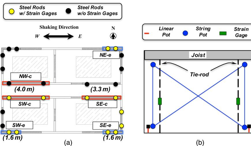
**Fig. 4.** Shear wall instrumentation plan: (a) location of instrumented shear walls typical of Levels 1, 2, and 4 (wall length specified in the parenthesis); and (b) typical shear wall sensor configuration.
