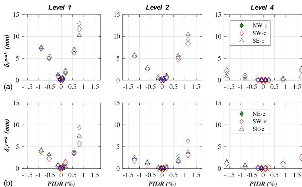
**Fig. 11.** Peak wall end vertical displacements of the (a) corridor; and (b) corner shear walls during the prefire earthquake test sequence.
