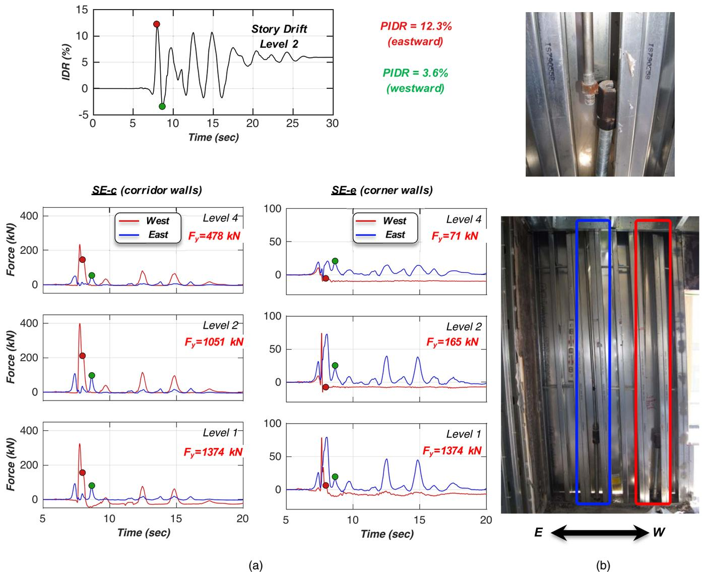
**Fig. 12.** (a) Tie-rod axial force histories of the southeast corridor and corner shear walls (SE-c and SE-e) during the postfire MCE test (EQ9); and (b) corner shear wall tie-rod (SE-e) connection failure at the end of the test program. Circles denote the time instances of the Level 2 peak story drift in the positive (eastward) and negative (westward) directions. The arrow indicates the direction of shaking (images by Xiang Wang).
