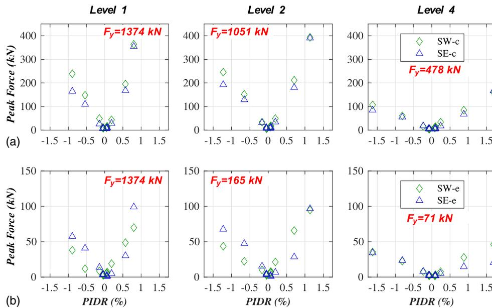
**Fig. 10.** Peak tie-rod tensile forces of the (a) corridor; and (b) corner shear walls during the prefire earthquake test sequence.
