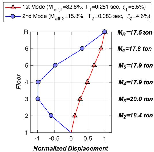
Fig. 14. Modal properties of the first and second longitudinal modes identified using the white-noise data recorded at the beginning of the earthquake test phase.
