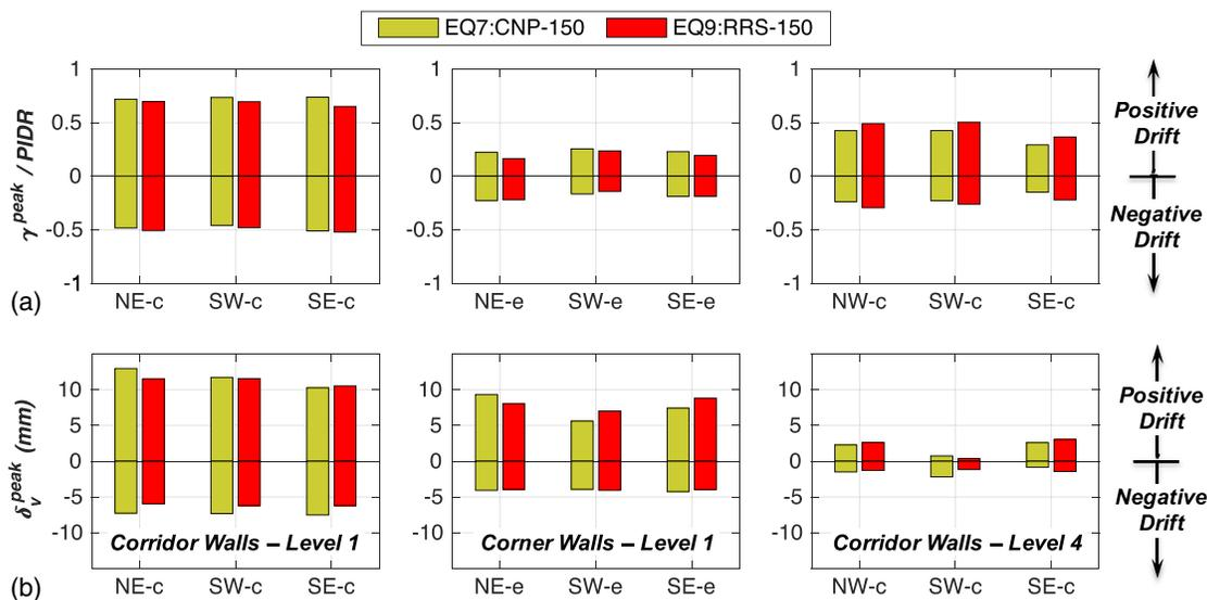
**Fig. 13.** Comparison of (a) peak sheathing panel shear distortion ratios; and (b) peak wall end vertical (uplift) displacements of select shear walls during the prefire and postfire MCE level tests (EQ7 and EQ9).
