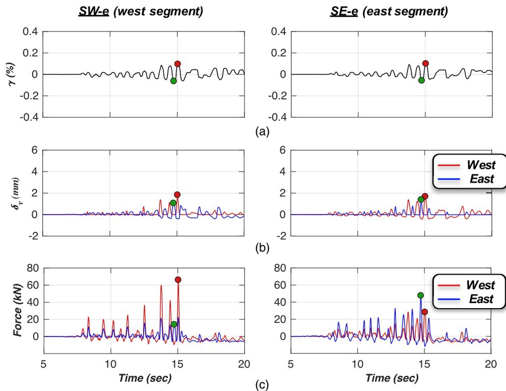
**Fig. 7.** Local responses of the longitudinal corner shear wall pair at Level 2 during the design event (EQ6): (a) panel shear distortions; (b) wall end vertical displacements; and (c) tie-rod axial forces. Circles denote the time instances of the Level 2 peak story drift in the positive (eastward) and negative (westward) directions (red-positive; green-negative).
