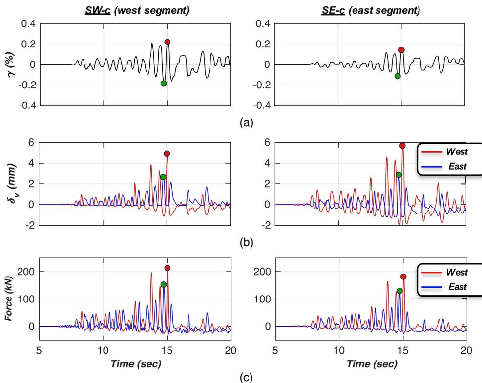
**Fig. 6.** Local responses of the corridor shear wall pair at level 2 during the design event (EQ6): (a) panel shear distortions; (b) wall end vertical displacements; and (c) tie-rod axial forces. Circles denote the time instances of the Level 2 peak story drift in the positive (eastward) and negative (westward) directions.
