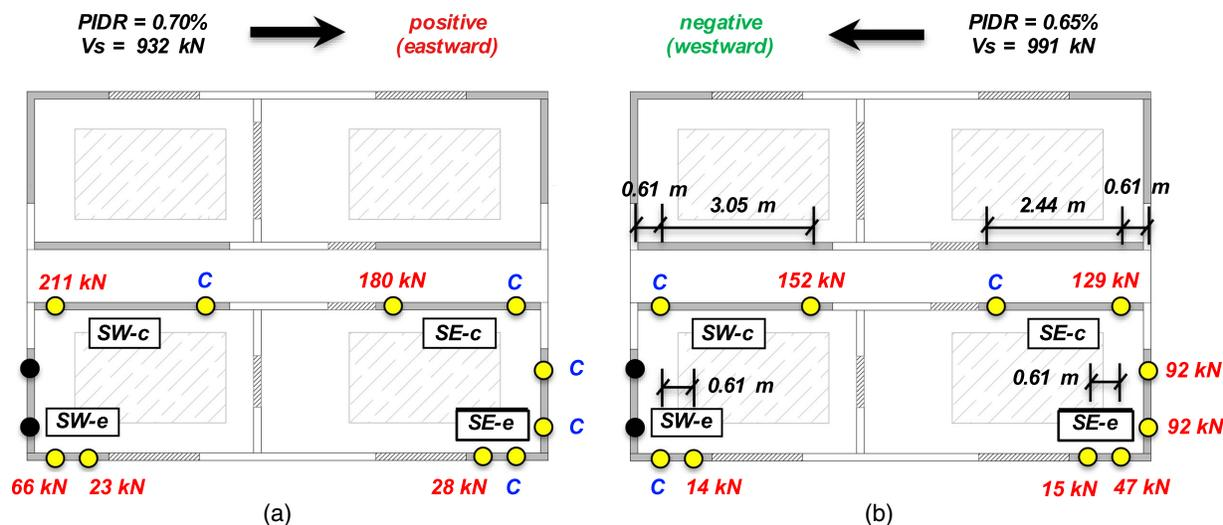
**Fig. 8.** Tensile force distribution of the Level 2 shear wall tie rods during the design event (EQ6): (a) positive peak story drift; and (b) negative peak story drift. C denotes that the tie rod was subjected to compression. Note that the tie rods of the transverse walls at the southwest corner were non-instrumented.
