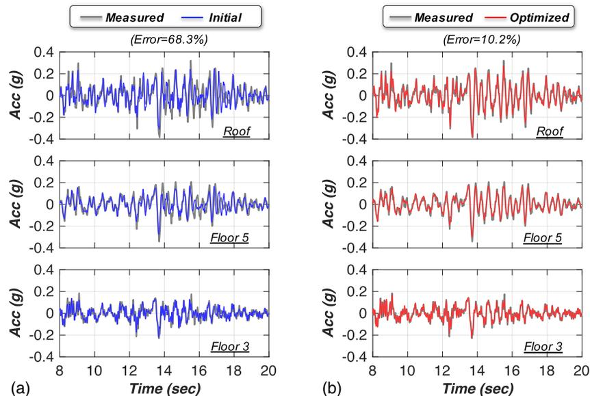
**Fig. 15.** Comparison of the measured floor accelerations of the test building during Test EQ2 and the modal superposition results simulated using (a) initial modal parameters; and (b) optimized modal parameters.
