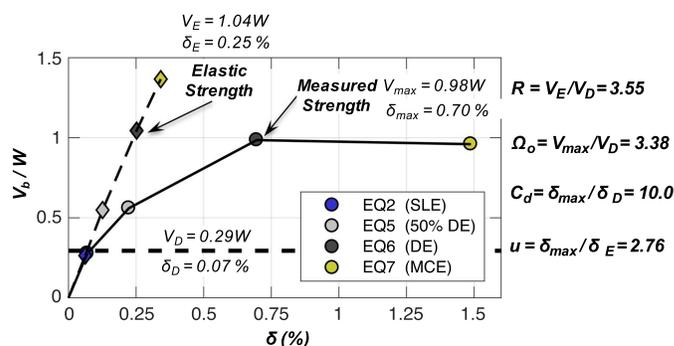
**Fig. 18.** Determination of key seismic design factors using measured peak roof drift ratio versus normalized base shear ( $V_b/W$ ) responses (solid line) during the four select earthquake tests with the corresponding linear responses (dashed line).
