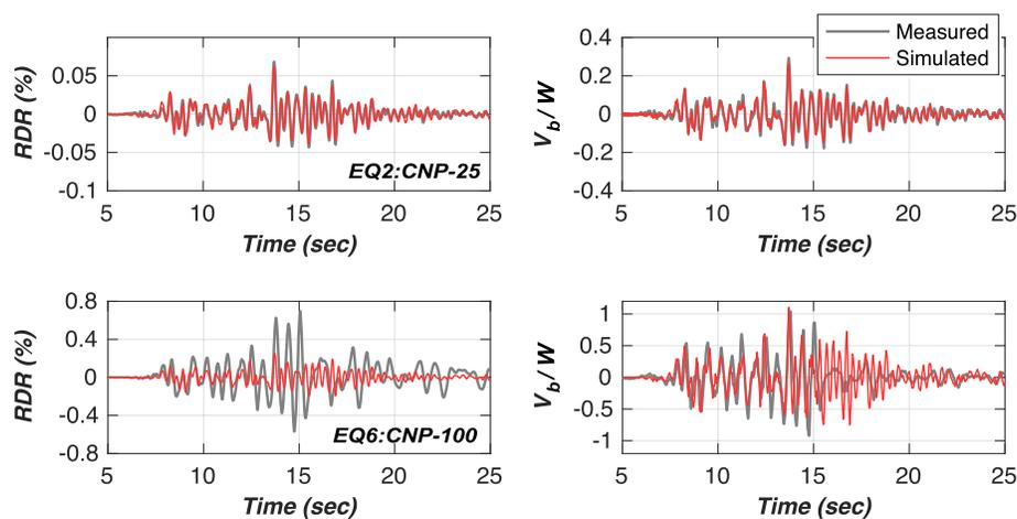
**Fig. 17.** Comparison among measured roof drift ratio, normalized base shear ( $V_b/W$ ), and simulated linear responses during Tests EQ2 (service level) and EQ6 (design level).
