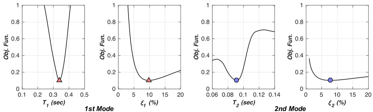
**Fig. 16.** Sensitivity of the objection function (RRMSE between the measured and simulated floor acceleration responses) with respect to the optimization parameters for Test EQ2. RRMSE denotes relative root-mean square error.
