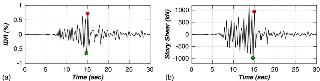
**Fig. 5.** (a) Level 2 story drift; and (b) story shear responses during the design event (EQ6). Circles denote the time instances of the Level 2 peak story drift in the positive (eastward) and negative (westward) directions.
