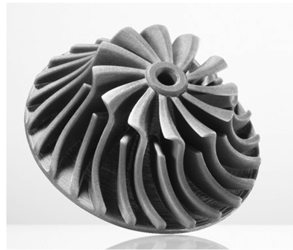
Fig. 20. \beta -SiAlON impeller created by Digital Light Processing after de-binding and sintering. The features indicate a part built to net shape that is not easily fabricated by conventional ceramic processing or machining techniques. The diameter is approximately 45 mm.
