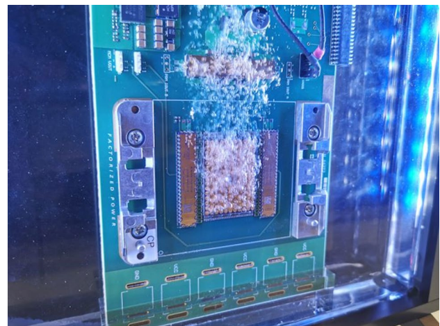
Fig. 26 Two-phase immersion cooling of electronic devices via nucleate boiling
