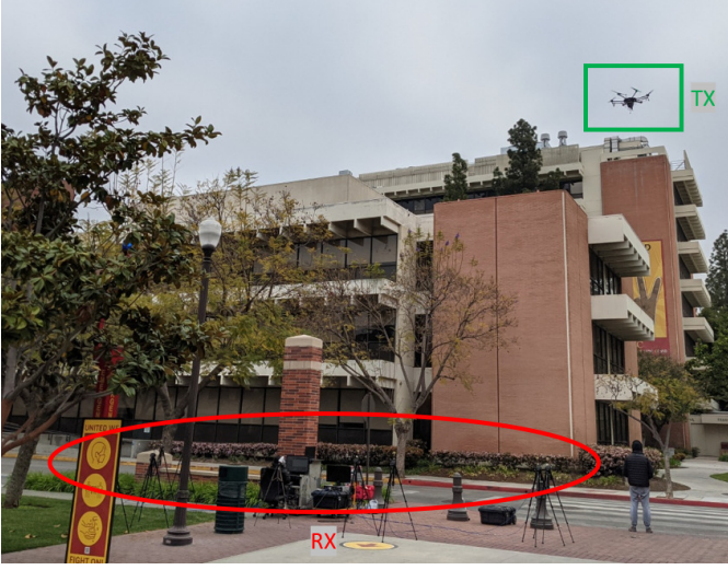
Fig. 2. Channel sounder setup: a single TX antenna on a drone passes through a trajectory containing all possible AP locations while 8 separated RX antennas on the ground are positioned at 8 different UE locations
