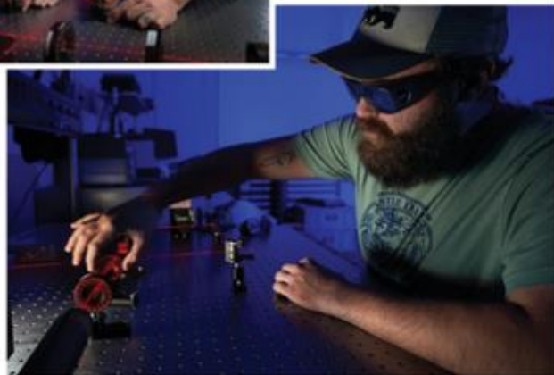
Students Arise Crawford and LeRoy Verwolf line up an experiment to determine the polarization extinction ratio of a polarizing beamsplitter (left). Student Christopher Long characterizes the properties of a polarizing beamsplitter (below).
