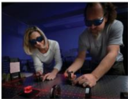
Students Arise Crawford and LeRoy Verwolf line up an experiment to determine the polarization extinction ratio of a polarizing beamsplitter (left). Student Christopher Long characterizes the properties of a polarizing beamsplitter (below).
